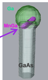
HAADF tomography Tilt range: +65° to -65° Increment: 2°
