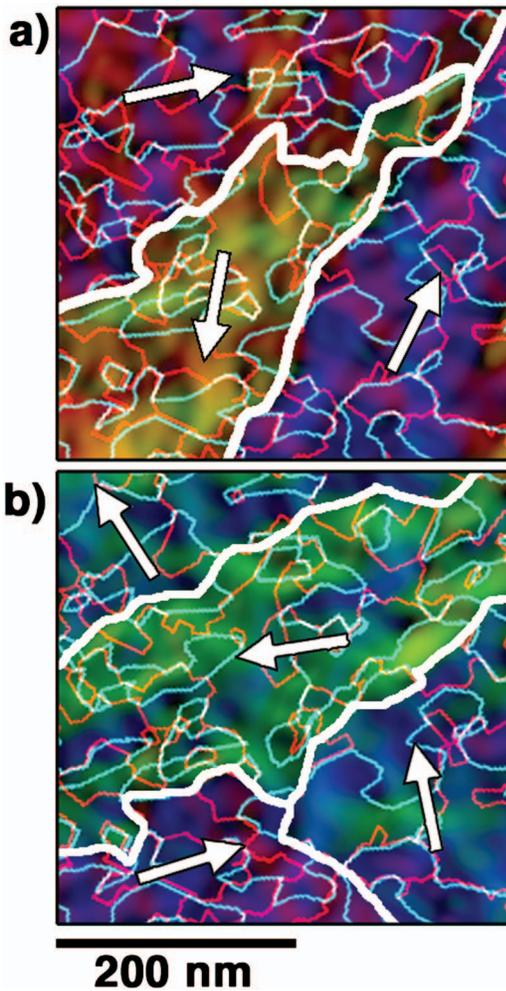
FIG. 5. (Color) Magnetic induction maps recorded using off-axis electron holography after applying in-plane fields of (a) +1048 and (b) -192 Oe, corresponding to Figs. 3(d) and 3(g). The boundaries of coarse magnetic domains are marked. Arrows indicate the average magnetization direction in each coarse domain.
