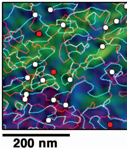
FIG. 9. (Color) Distribution of APB's that have magnetic moment angles of  $>70^\circ$  from the film plane, after applying an in-plane field of  $-192$  Oe to the specimen. The white solid circles correspond to antiferromagnetic coupling at APB's, while the red solid circles correspond to antiferromagnetic coupling away from the positions of known APB's.
