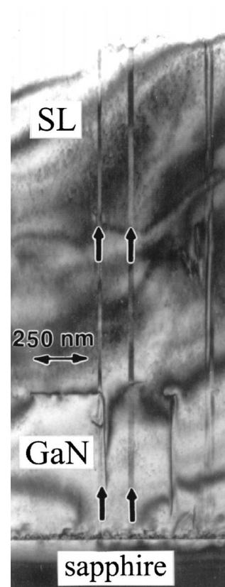
FIG. 1. Cross section of the sample with a superlattice in the top region. Arrows mark two inversion domains which originate in the GaN buffer layer and traverse through the whole layer to the top surface.
