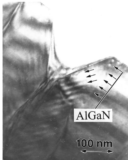
FIG. 5. AlGaIn/GaN superlattice (with a periodicity of 30 nm) bent around a V pit. The image is taken at two beam condition to show the bent layers clearly, while the walls of the inversion domain are not sharp at this tilt.
