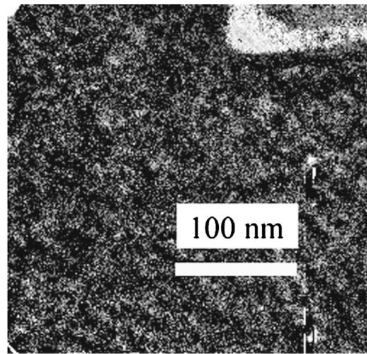
FIG. 4. Chemical map showing Al at a pit on the surface of an AlGaIn/GaN superlattice.
