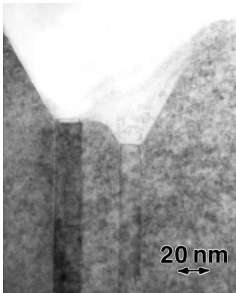
FIG. 3. High-resolution image of a pit formed on the surface of an AlGaIn/GaN superlattice.
