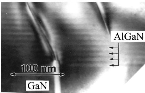
FIG. 2. High magnification image of AlGaIn/GaN superlattice grown on GaN.
