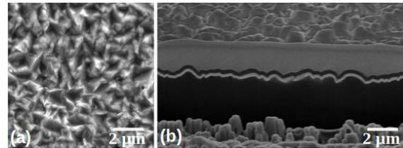
Fig 4: (a) Top view back reflector and (b) FIB cross-section of roll-to-roll scale a-Si SEM images
