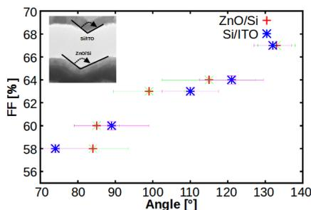
Fig 3: Fill factor as a function of opening angle measured at the ZnO/a-Si and Si/ITO interfaces. Insert shows how the angles have been measured.
