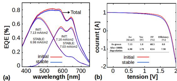
Fig 6: (a) spectral response and (b) IV curve of the tandem cell obtained at reference cell. The values in the table are average over 10 different cells.
