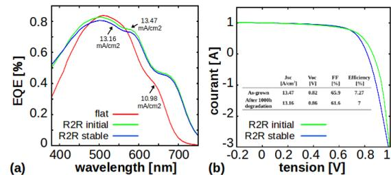
Fig 5: (a) spectral response and (b) IV curve of the cell obtained in roll-to-roll for flat and UV embossed texture.
