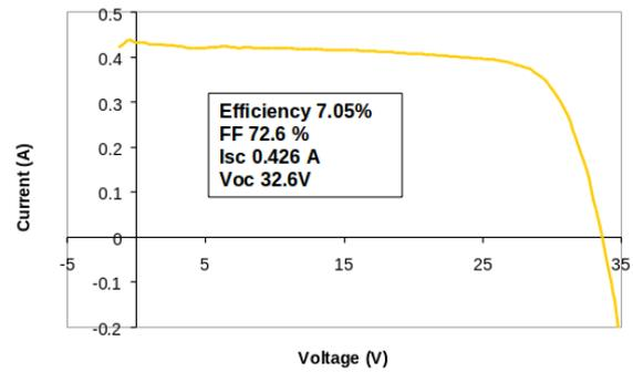
Fig 8: IV curve of the module tandem cell obtained by roll-to-roll process on plastic substrate. The initial electrical performances are shown in insert.
