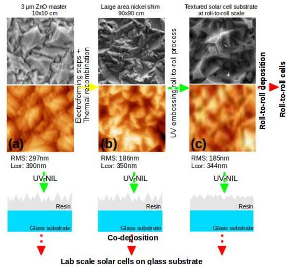
Fig 1: Process flow used to produce textured substrates. The (a) type 1: original 3  $\mu$ m thick ZnO layer, (b) type 2: large scale nickel mold and (c) type 3: textured plastic substrate is used as molds to transfer the texture to the glass substrates. The textures are transferred to the glass/plastic substrates by UV-NIL embossing. Then, solar cells are grown on textured substrates. All the AFM and SEM images are at the same scale.
