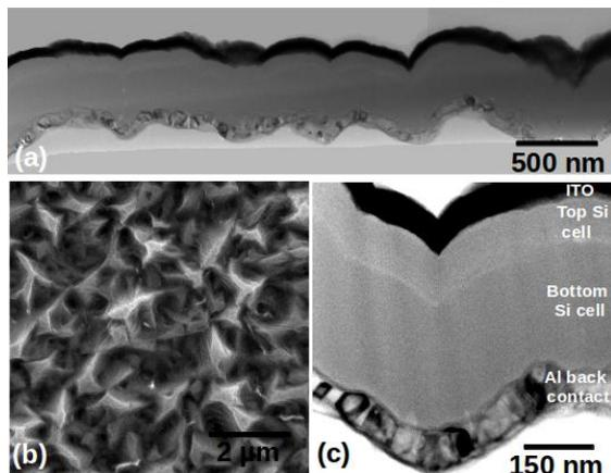
Fig 7: (a)-(c) cross-section TEM images of the a-Si tandem cell on plastic foil. (b) top view SEM images of textured plastic substrate by roll-to-roll process.
