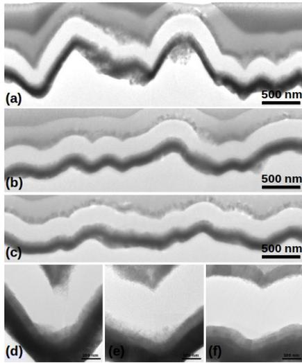
Fig 2: TEM pictures of solar cells grown on textured substrates, obtained from the (a)-(d) type 1, (b)-(e) type 2 and (c)-(f) type 3. From the bottom to the top, the layer stacking is: resin, Ag, ZnO, a-Si and ITO.
