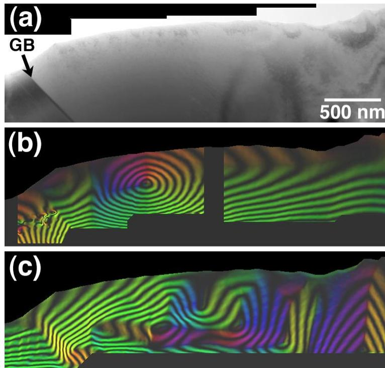
**Figure 2.** (a) Bright-field TEM image of a synthetic magnetite specimen with a grain size of 10-30  $\mu\text{m}$ , which was prepared for TEM examination using Ar ion milling. (b, c) Remanent magnetic states recorded using off-axis electron holography from the same region at room temperature and below the Verwey transition, respectively. The phase contour spacing is  $2\pi$  radians. The location of grain boundary (GB) is marked in (a).
