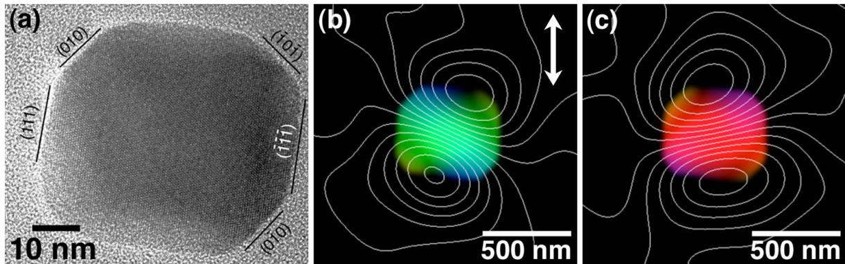
**Figure 1.** (a) High-resolution TEM image of a 50-nm-diameter magnetite crystal from a magnetotactic bacterial cell (recorded by M. Pósfai). (b, c) Remanent magnetic states recorded from the same particle using off-axis electron holography at room temperature and at 90 K, respectively. The double arrow in (b) shows the direction of the in-plane component of the applied field before reducing the applied field to zero and recording electron holograms.
