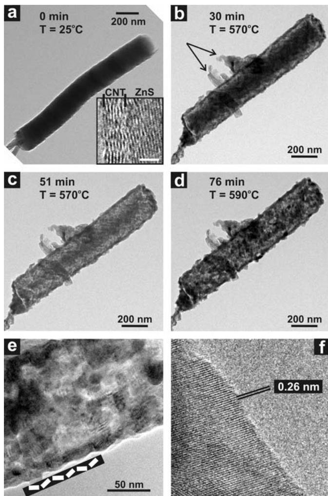
FIG. 1 (a) Bright-field TEM image of a thick, low-aspect-ratio  $\text{Zn}_{0.92}\text{Ga}_{0.08}\text{S}@\text{CNT}$ . Inset: detail of the sulphide core – carbon shell region. Scale bar: 2 nm. (b) to (d) Different stages of the structure during in-situ TEM oxidation. The arrows in (b) indicate unexpected foreign structures. (e) Detail of (d) highlighting the faceted nature of the thick external wall. (f) High-resolution image of an oxide grain on the external wall of (d).
