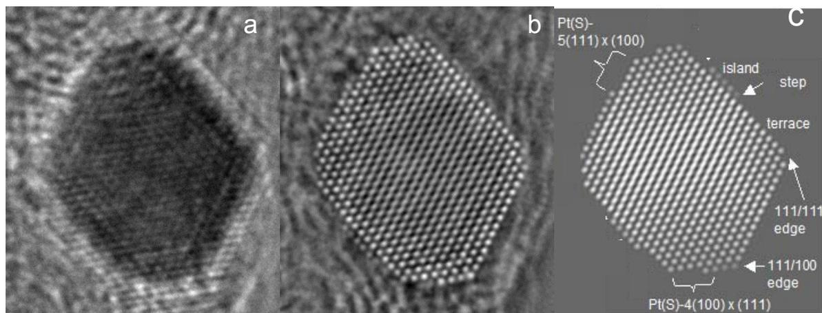
FIG. 1. (a) High-resolution image of a platinum particle supported on carbon in the [110] zone-axis. (b) Restored phase of exit plane wavefunction from a focal series of 20 images acquired at 200kV with  $C_s$  adjusted to  $-4 \mu\text{m}$ . Islands and steps on the surface of the nanoparticles are clearly resolved. (c) Phase of exit plane wavefunction simulated using multislice method, from the model which is best fitted with the experimental restored phase shown in (b).
