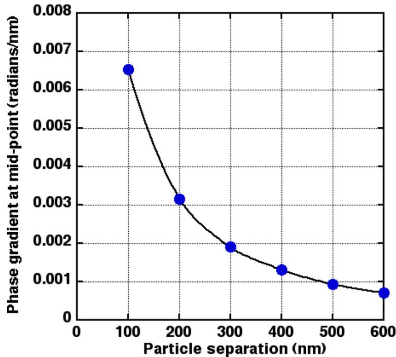
**Figure 4.** Phase gradient measured from micromagnetic simulations such as those shown in the lower part of Fig. 3, measured mid-way between two collinear ellipsoidal  $36 \times 300$  nm ferromagnetic Fe nanoparticles as a function of their separation.
