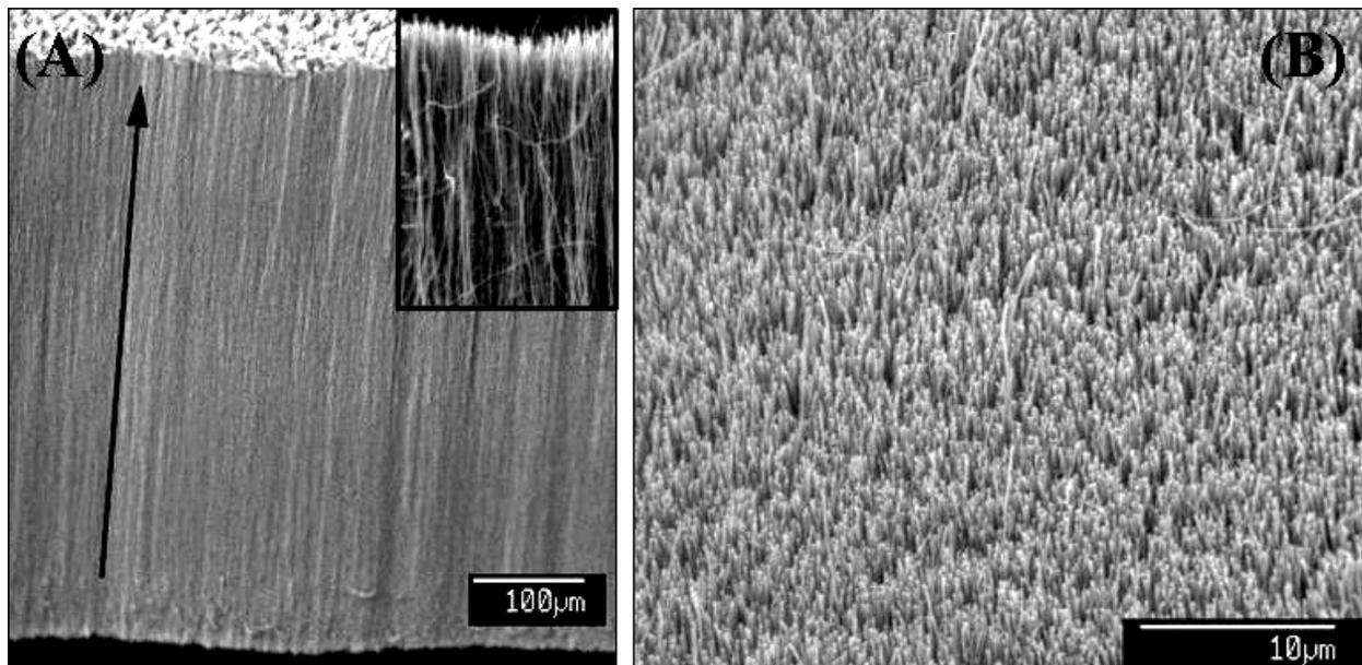
**Figure 1.** Scanning electron micrographs showing (A) side and (B) top views of aligned carbon nanotube arrays that contain encapsulated ferromagnetic iron nanoparticles. The nanotube density of  $5 \times 10^6 \text{ mm}^{-2}$  is determined by the synthesis conditions used. The arrow in (A) indicates the direction of nanotube alignment.
