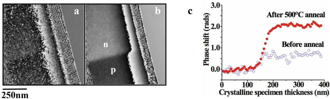
FIG. 1. Wrapped holographic phase images of a FIB-milled GaAs *p-n* junction of crystalline thickness 240 nm, recorded at room temperature (a) before and (b) after *in situ* annealing at 500 °C. (c) Phase profiles measured across a FIB-milled GaAs *p-n* junction in a sample of crystalline thickness 300 nm, before (open circles) and after (closed circles) annealing at 500 °C.
