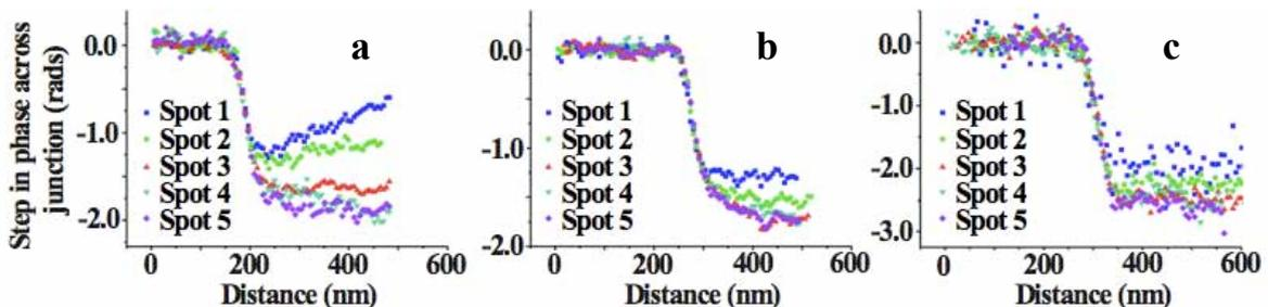
FIG. 2. (a) Phase profiles across a GaAs *p-n* junction of crystalline thickness 320 nm. (b) Profiles of the same specimen acquired after C coating. (c) Profiles acquired with improved electrical contacts applied to the specimen in a biasing holder.
