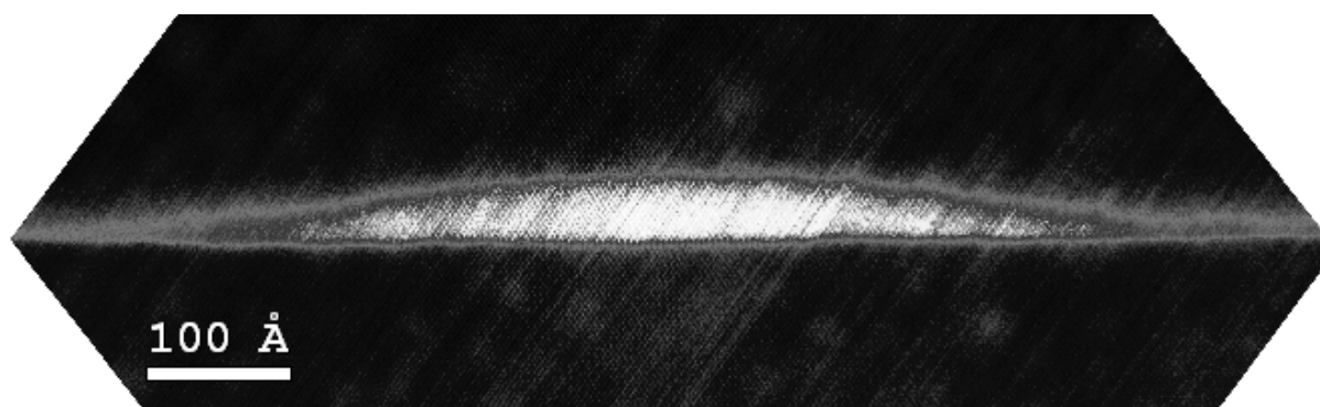
Figure 4. Z-contrast STEM image of a buried Ge QD.
