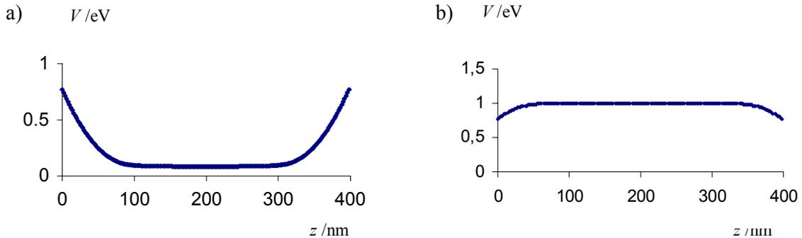
**Figure 3.** Simulated potential energy along a) line 'b' and b) line 'c' in Figure 1 (electron volts above the Fermi level), for a specimen of thickness 400nm.
