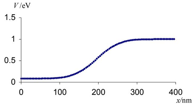
**Figure 2.** Conduction band energy (measured in electron volts above the Fermi level) along line 'a' in Figure 1. The dopant concentration is  $10^{17} \text{ cm}^{-3}$  for both the Sb-doped (*n*-type) and the B-doped (*p*-type) sides of the Si p-n junction.
