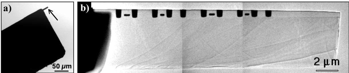
**Figure 3:** Bright field images of sample milled in several directions using FIB (final thinning from substrate side), with surface subsequently cleaned using low angle ion milling in a Gatan PIPS. Membrane is arrowed in a).
