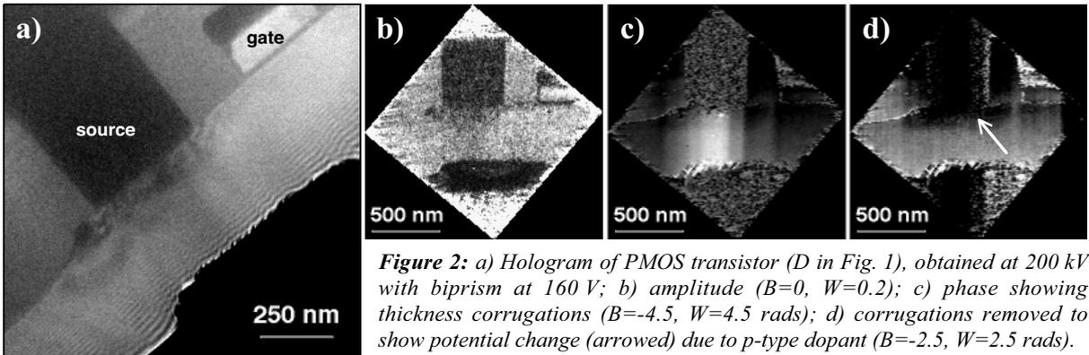
**Figure 2:** a) Hologram of PMOS transistor (D in Fig. 1), obtained at 200 kV with biprism at 160 V; b) amplitude ( $B=0$ ,  $W=0.2$ ); c) phase showing thickness corrugations ( $B=-4.5$ ,  $W=4.5$  rads); d) corrugations removed to show potential change (arrowed) due to p-type dopant ( $B=-2.5$ ,  $W=2.5$  rads).
