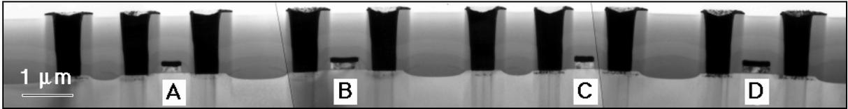
**Figure 1:** Transistor sample prepared by FIB. A, B, C and D are NMOS (0.35 μm gate), NMOS (0.5 μm gate), PMOS (0.35 μm gate) and PMOS (0.5 μm gate) transistors, respectively.
