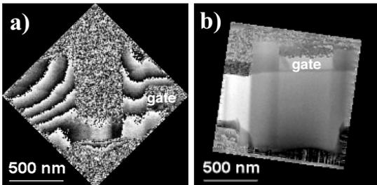
**Figure 4:** (Wrapped) phase images of identical transistor to that shown in Fig. 2, both obtained at 200 kV with a biprism voltage of 140 V. a) Sample of thickness 340 nm, examined before depositing carbon onto it to prevent charging; b) Sample of thickness 100 nm. No contrast is visible at the position of the p-type dopant because the combined thickness of the surface depletion layers at the top and bottom surfaces of the sample is comparable to the total sample thickness.
