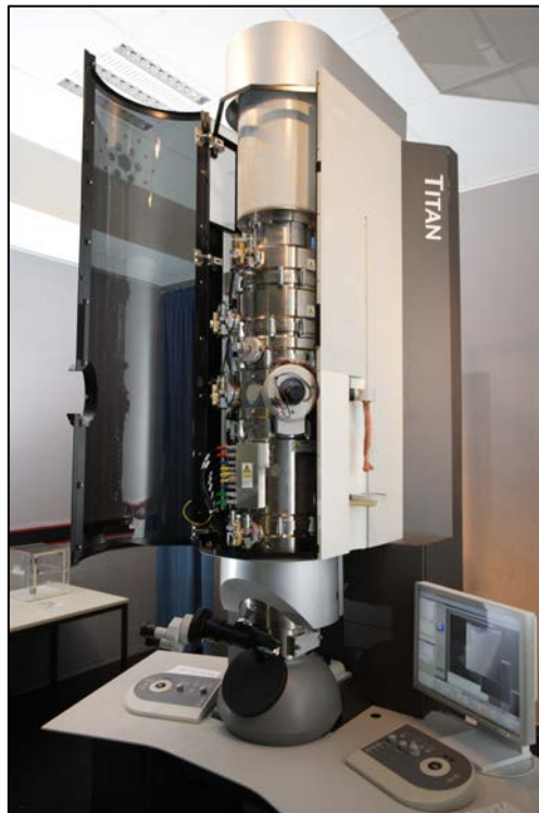
Fig. 1: FEI Titan 80-300 field emission transmission electron microscope at Forschungszentrum Jülich. The instrument is equipped with a spherical aberration corrector on the objective lens and has an information limit of 0.08 nm
