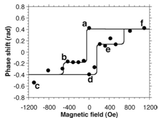
Figure 4 Remanent hysteresis loop measured directly from the experimental electron holographic phase images, with the letters corresponding to the six individual figures shown in Fig. 3. The graph shows the magnetic contribution to the phase shift across each element, plotted as a function of the in-plane component of the field applied to the elements before recording the remanent states. Each point shows an average of the phase shifts measured from the three elements shown in Fig. 3.
