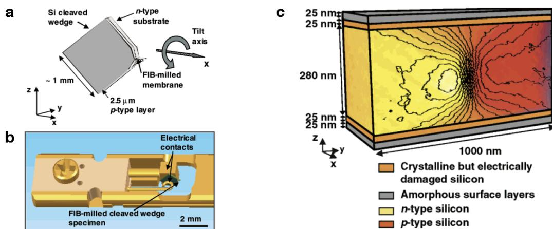
Figure 5. (a) Specimen geometry used for electrically biased tomographic holography. (b) Drawing of a two-contact electrical biasing TEM specimen holder. (c) Tomographic reconstruction of the electrostatic potential in a focused ion beam milled specimen containing an electrically biased Si  $p-n$  junction. Contours spaced every 0.2 V have been superimposed onto the reconstructed tomogram.
