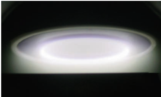
FIG. 2: Photograph of plasma and target holder with a YBCO target and a MACOR insulator during the high oxygen pressure magnetron sputtering.
