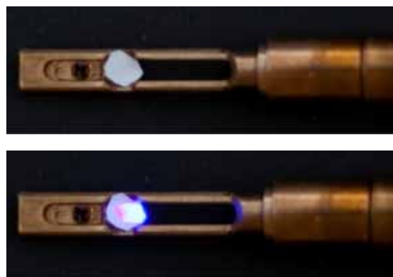
TEM holder with in-situ light emission capability.
